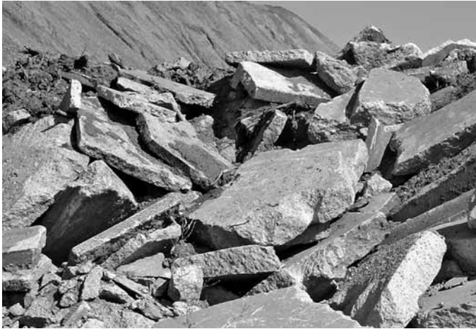
This material makes excellent base aggregate. The material is being crushed and processed at Brown County Highway Department. Note the various concrete products that are being recycled.
